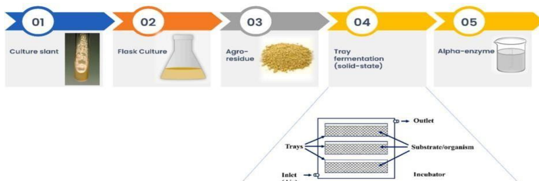
Figure 4. Stages of solid-state fermentation in \alpha -amylase production from agro-industrial substrates (Sahu et al., 2024)
